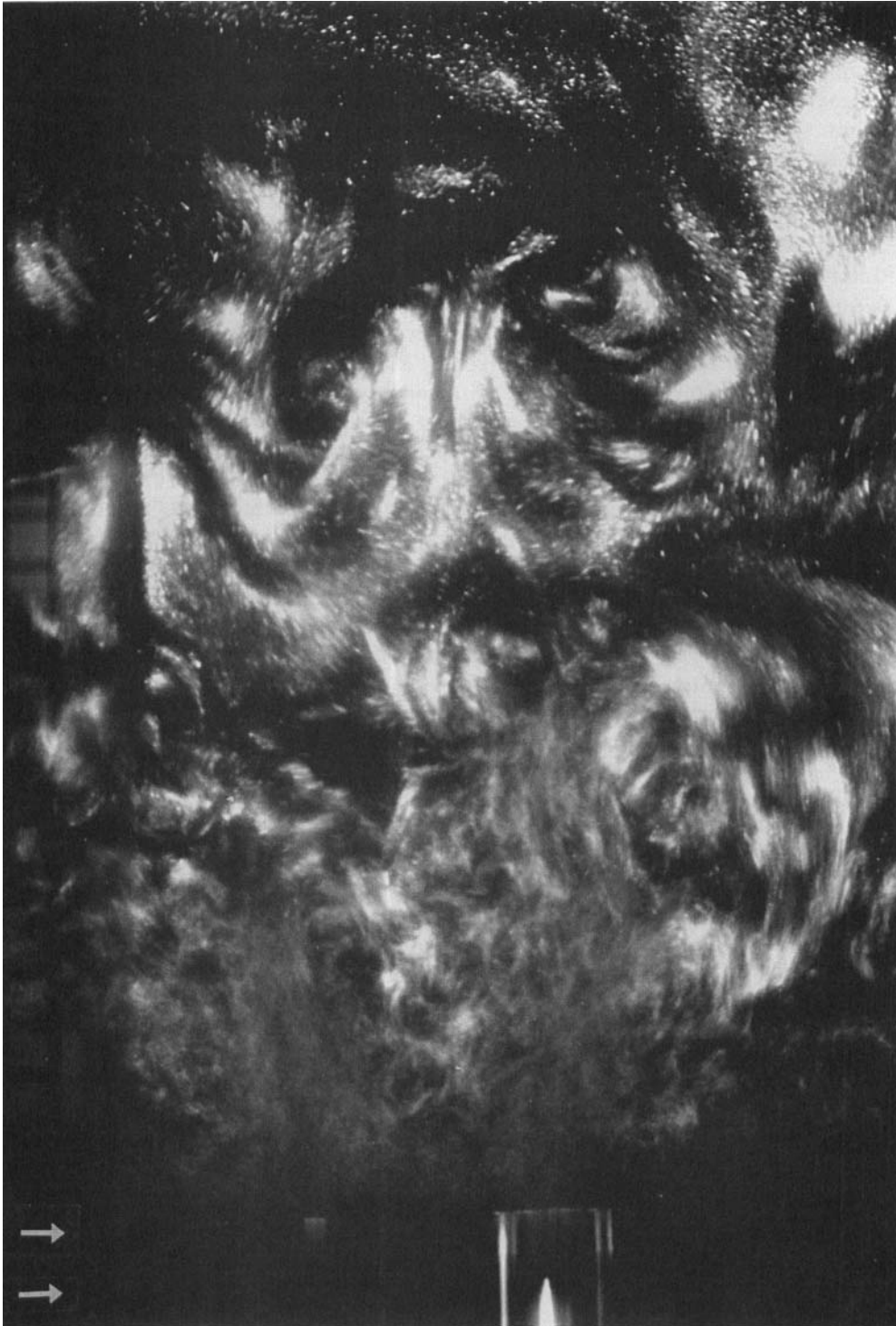
FIGURE 5. The turbulent motions generated by the grid, with a 2.4 cm stroke and frequency of 4 Hz, in a homogeneous fluid seeded with fish scales and illuminated through 1 cm wide slits. Regions of strong turbulent activity, in the form of turbulent wakes, can be seen near the grid, extending approximately 10 cm from the virtual origin. The divisions on the left of the photograph are at 1 cm intervals. The bottom arrow on the left of the photograph marks the grid's mean position and the top arrow identifies its position at the top of its stroke. The photograph was taken with a 1 second exposure.
